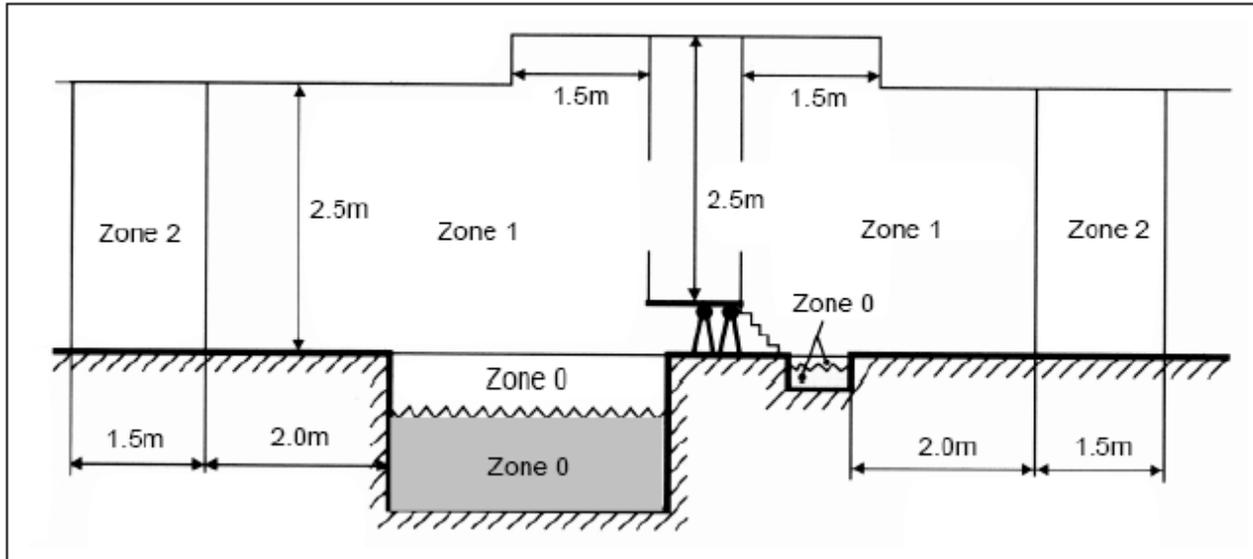
NOTE: The measured zone dimensions are limited by walls and fixed partitions. Above figure--Zone dimensions of swimming pools and paddling pools.
