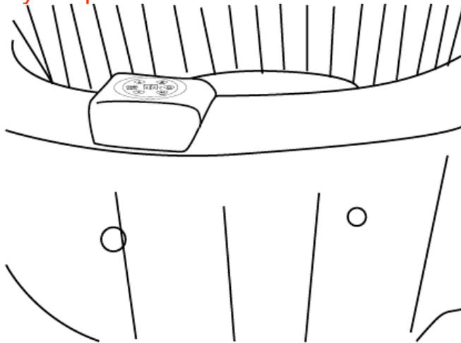
1. Water filling of water tank body: water should be filled to a position 20mm higher than the water line. If lower, heating may not be realized. If higher, water may spill over the tank in use.
