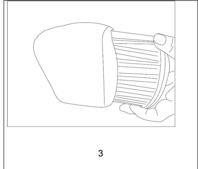
4. The filter cartridge can be rinsed off with a garden hose and reused. However, if the filter cartridge remains soiled and discolored the filter cartridge should be replaced.
